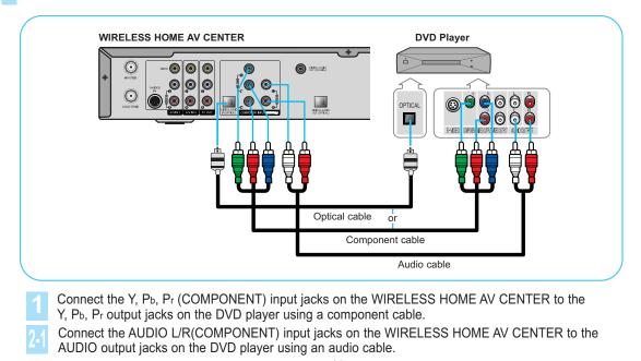
Connect the optical input jack on the WIRELESS HOME AV CENTER to the optical output jack on the DVD player using an optical cable.
